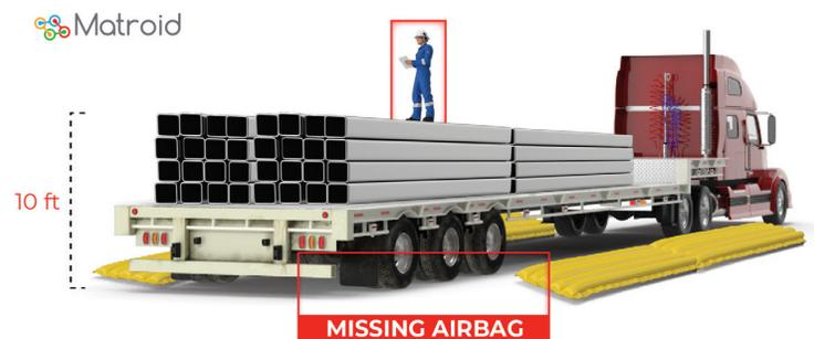
**WARNING:** Employee working at height near missing airbag
