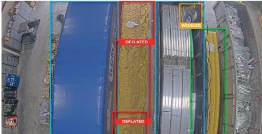
Figure 2. Matroid's computer vision platform can identify and alert for potentially damaged, deflated or missing airbags.
